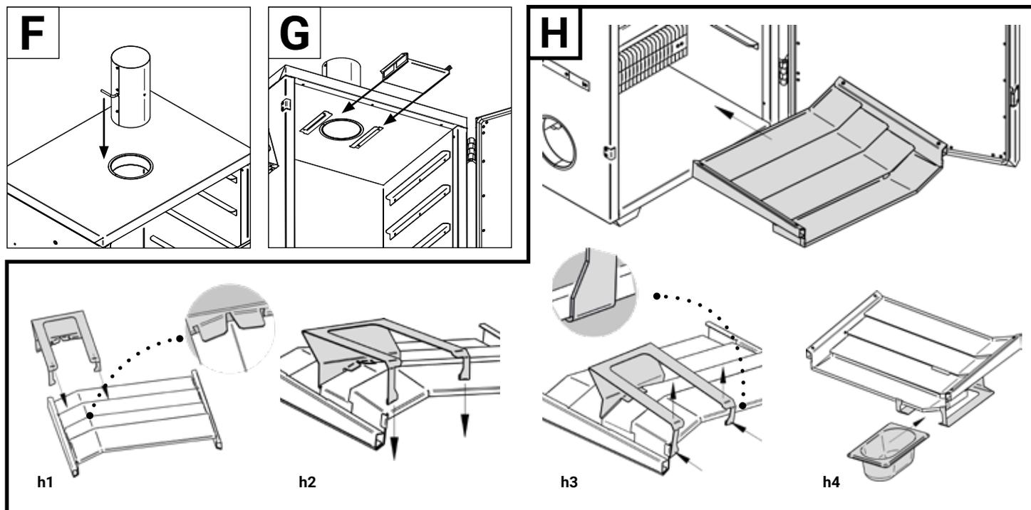
**H)** Install the drip tray holder before inserting the drip tray. To do so, turn the tray over and insert the hooks as shown in figure **h1**). Then attach the handle onto the edge of the tray as shown in figure **h2**) and **h3**). Turn the tray back over, place it in the smoker and insert the tray as shown in figure **h4**).
