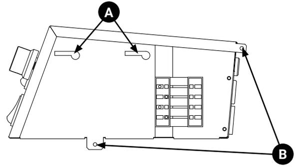
I) Loosen the screws (point **B**) from the smoker housing. Mount the electronic panel so that the holes in the panel align with the screws (point **A**). Slide the panel toward the back wall of the smoker until the connectors on the panel and smoker connect. Insert and tighten the screws in the correct locations (point **B**).
