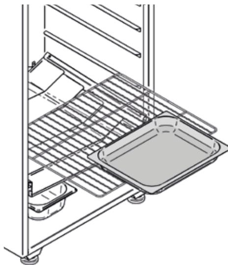
Correct positioning of the tray is shown in the figure above.
